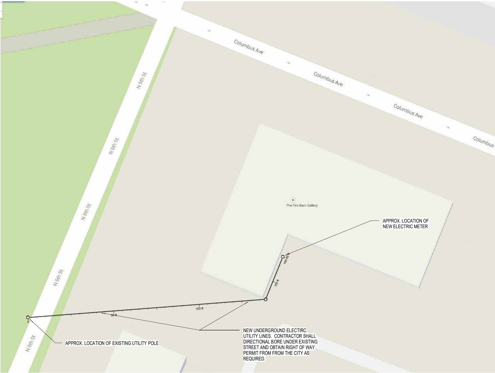
ANNEX ELECTRICAL SITE PLAN - ALTERNATE E-1
